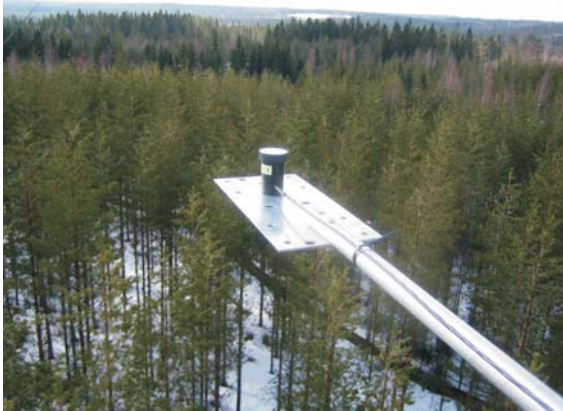
NDVI sensors on eddy covariance tower over forest canopy
