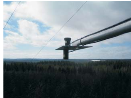
Pair of NDVI incident & reflected light sensors
