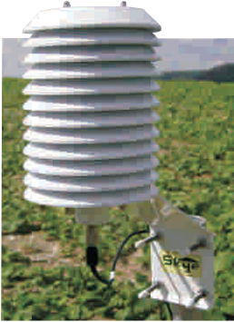
rht+ Probe mounted in a Radiation Screen
