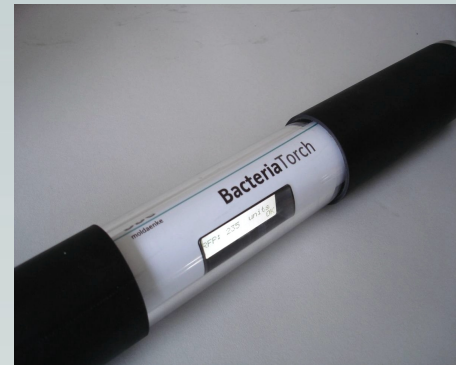
ABOVE: head with flow-through device BELOW: Bacteria Torch for rapid detection of RFP and GFP Fluorescence
